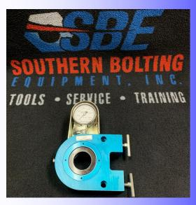
With the Skidmore MZ, you can accurately simulate join conditions, then transfer your tightening procedure to the joint itself. Your result is consistent tightening to bolt tension specifications. The Research Council on Structural Connections recommends a tension measuring devise such as the Model MZ be available at every job site. Obsolete torque checking methods will not let you meet approved bolt tension specifications.
